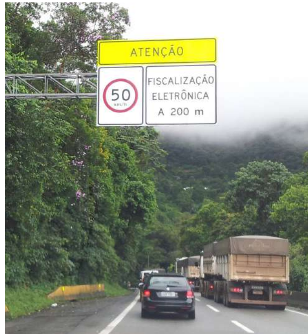
Image 5. Bad-practice signposting for speed cameras and highly visible cameras: informing drivers of exact enforcement locations
