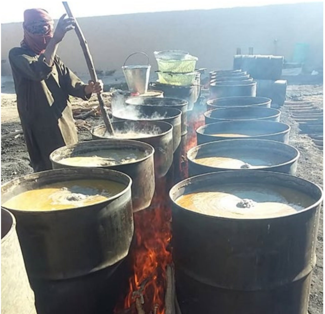
Figure 9. Ephedrine/pseudoephedrine from plant origin being extracted and processed by boiling in liquid at an industrial scale in Western Afghanistan.
