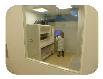
During 2019, the Laboratory procured the instrumentation required for this analysis and, with the support of the Office of Public Works, upgraded one of its laboratories to provide the necessary controlled temperature and humidity environment required for the correct operation of a smoking machine. Once the
